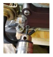
Here is the screw hole being drilled using the kit-supplied drill bit mounted in an electric drill.
