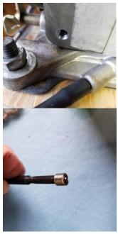
After tapping the hole, I used another blast of compressed air to blow out any aluminum chips. I then removed the alignment fixture.
