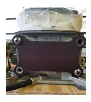
Here is the alignment fixture mounted to the carburetor main body. To prevent metal chips from clogging passages in the carburetor, I placed masking tape over all of the holes in the mounting surface of the main body before installing the fixture. I also covered the top opening of the carburetor (air horn). I have the small bushing positioned over the lower left hole in preparation for drilling.
