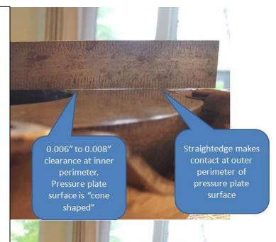
Placed straightedge across pressure plate contact surface. Inner perimeter has a gap ranging from .006 to .008" all around.
