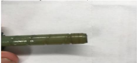
You can see the faint black line at the far right end of the gear stem. I should not have been surprised since I know how a lip seal can grove a crankshaft.
