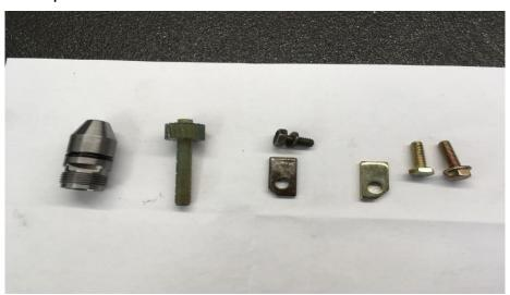
Here is a picture of the old adaptor, driven gear and old hold down hardware. The 3 pieces to the right came with new kit.
