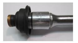
After the pump is disassembles, the new components installed and the pump re-assembled the system should pump water. In re-assembling the unit make sure the four screws are tightened evenly to insure the "O" ring gaskets are seated properly.
