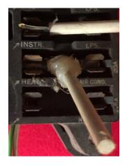
I cut the dowel the length of a fuse, glued a small piece of sandpaper onto the dowel with the hot glue gun, then cut a piece of dowel approximately 2". Made a "T" with the two pieces, glued them together and went to work.
