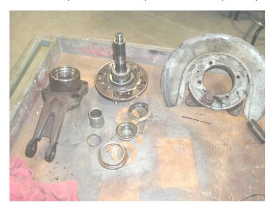
Here I found someone was in here before and installed the outer seal backwards.
