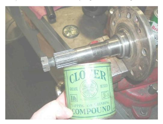
The spindles are cleaned up, the arms painted, bushings installed, and bearing endplay set. One of the spindle preps I do is to remove the rivets and tap the hole 3/8-24. We'll explore this more when I get to the rotors.
