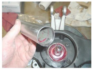
Grease the inner bearing and put it on the spindle. Transfer to the press again and press the inner bearing on the spindle. Bring it back to the bench and install the inner seal- again RTV on the OD. I then usually re-use the shield and loctite it in place. With the yokes, I again grind them, clean them up and chase the threaded holes.
