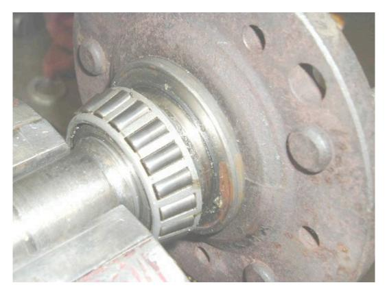
Once stripped down, I remove the front bushing
