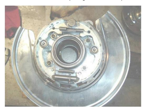
Now before you install the spindle you have to remove the outer bearing. This should be done before you get to this point. Remove the bearing, clean the spindle, check the journals, replace the studs and I face the flange in a lathe as well.
