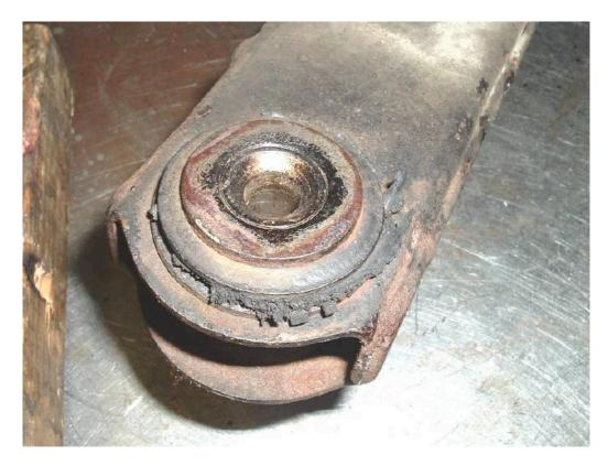
I use one of those spindle protectors and either press or hammer the spindle out. If you hammer them out place something to catch the spindle. Don't worry about the bearings as they will be replaced anyway. If you have one that is really rusted the press and some heat may be the only way to go. Also the spindle nut should come off and the tool thread on without a problem. Many times these have been worked on before and the threads are already shot and a new spindle is needed.
