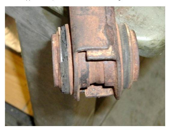
Drill the flare out and use an chisel to remove. I used to put these in a Bridgeport mill but a large step drill works as well.
