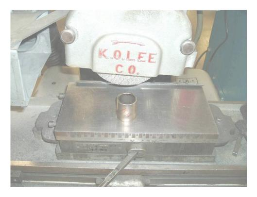
OK with the spacers ground and in the fixture. I use a large shim to start. I have one that I use as a setup shim. I torque the tool to 100 ft/lbs and see how much endplay I have. Then grind a new shim to size and double check it. I only use light spindle oil on the bearings- no grease until you are done and ready to install the bearing in the press.
