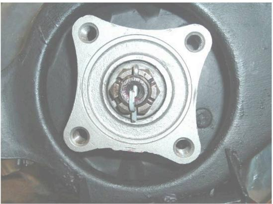
Torque the new nut to 100 ft/lbs and check the hole for the cotter pin. If needed you can tighten some more and install the new pin. If the hole is out a lot I grind the nut face to index it on the spindle. The spindle should spin snug but not tight. If you need two hands to rotate it there is something wrong. At .002 endplay you can feel
