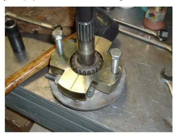
Now if the threads are rolled a little you may be able to save them. I have a thread forming tool, thread file, lathe, but you can use the "old school way" of using an old nut and some very fine lapping compound to clean them up. BE sure the threads are good and you use a new nut before you get to the bearings.
