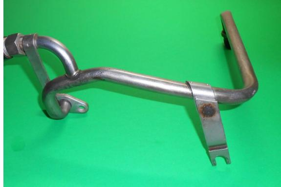
Eastwood carries a good quality 3/8" spot weld drill bit. Clamping the pipe on my drill press allowed for accurate removal of the top of the spot weld without drilling through the bottom piece. This made it much easier to re-attach it with a couple of small tack welds
