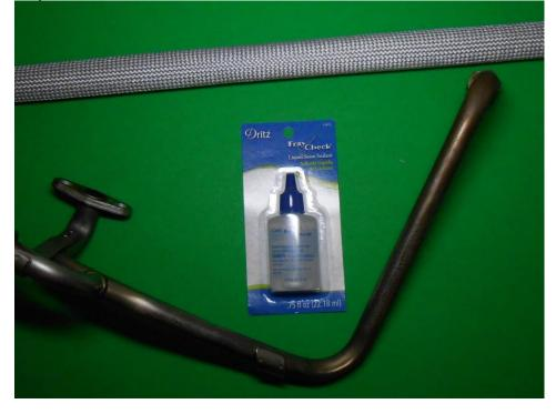
After the new sleeve material was cut to the proper length and the fray check applied it was slipped over the pipe. The slot for the bracket was cut in the sleeve the length of the tab at that time with a sharp razor. I put fray check on both sides of that cut, too.
