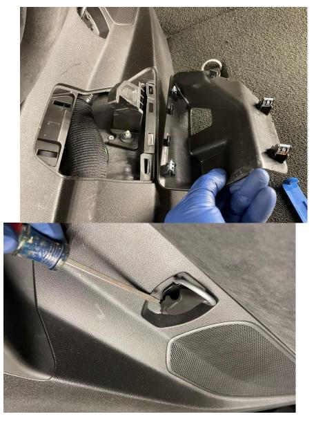
more sq. feet than you think you'll need. I'll explain later. To remove the cargo deck carpet you will need to remove both side rear interior panels. Using a pick and small screwdriver, remove the cover over the hardtop retainer bracket, this has 4 clips. Then take the small screwdriver pop off the "D" hook cover. This will allow you access to the 40mm torx that holds the ring in place.
