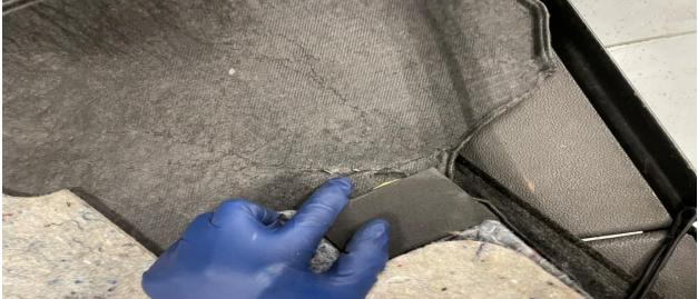
Now you can test fit the foil barrier, making marks and adjustments with a felt marker and trimming with a sharp blade or scissors. Another note is to be careful; the foil edge is very sharp as my right
