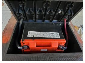
Once the top was cut free, I removed the bolts from the cables at the AGM battery and removed the battery case cover. I left the cables attached to the underside of the battery cover posts.
