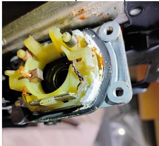
I found a used brush/spring assembly on the internet for \$11. After replacing the corroded spring and reassembly, the motor works great.
