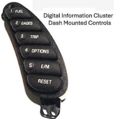
The C5 Corvette has the ability for users to pull any stored engine codes from the DIC on their dash. Users can also navigate the code(s) stored by the system, see the state of the code, and reset codes if they choose. It's user friendly and incredibly useful, but there are a few tricks to know.
